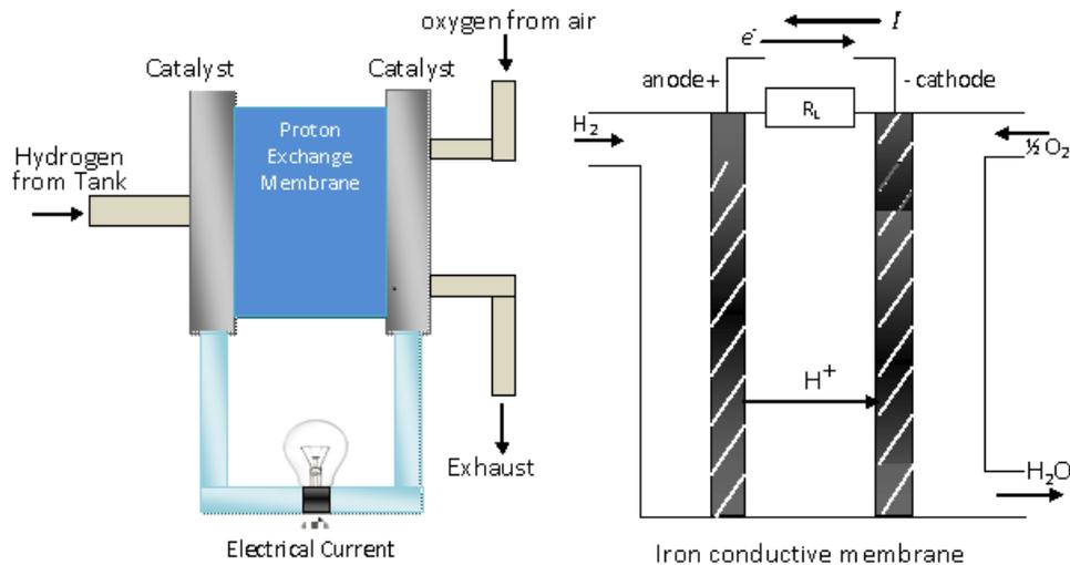
**Figure 1:** Basic Operating Principle of Fuel Cell
