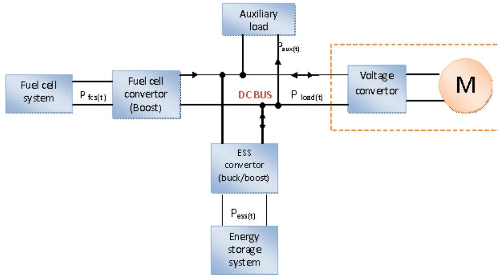
**Figure 2:** Diagram showing the electrical topology and the power flow in a Fuel Cell Hybrid System
