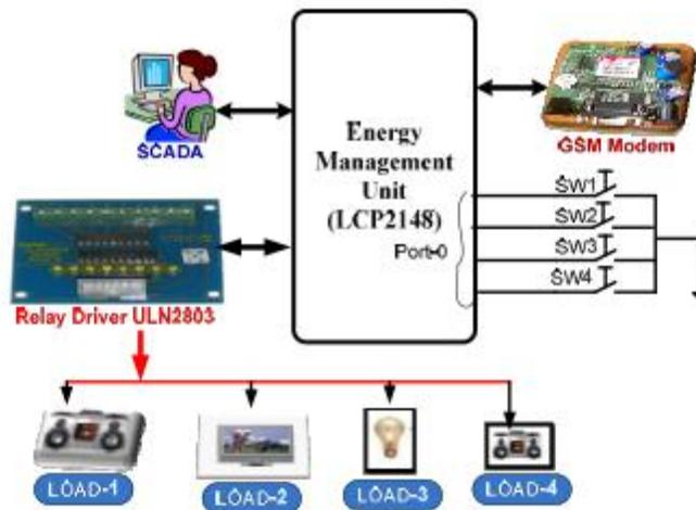
**Figure 1.** Schematics of Energy Management System
