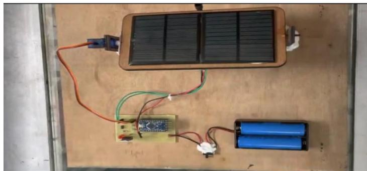
**Figure 9:** Snapshot of miniature solar tracker
