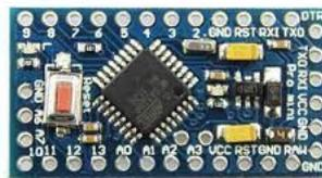
**Figure 3:** Mini Arduino
