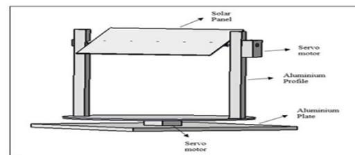
**Figure 2:** Dual Axis Solar Tracker
