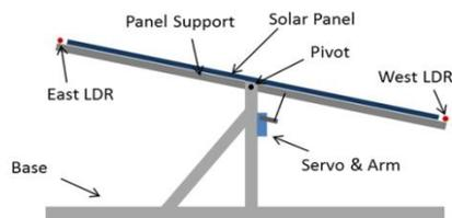
**Figure 1:** Single Axis Solar Tracker
