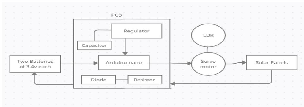
**Figure 8:** Circuit Diagram
