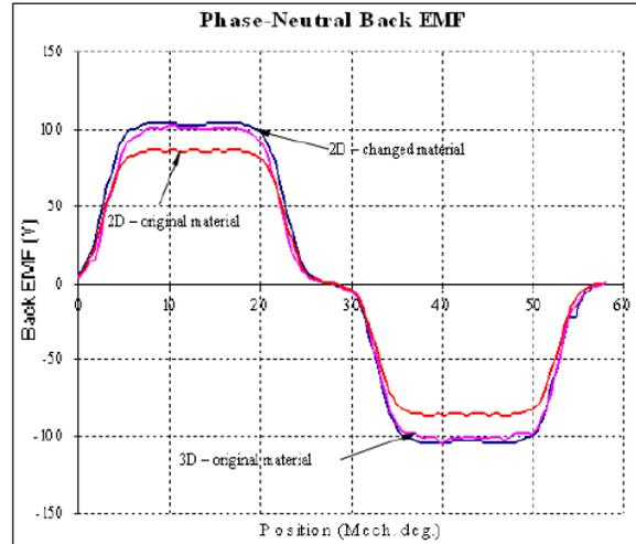
**Figure 9:** PM BLDC motor with 18 stator slots and 12 rotor poles has a phase-neutral back EMF.
