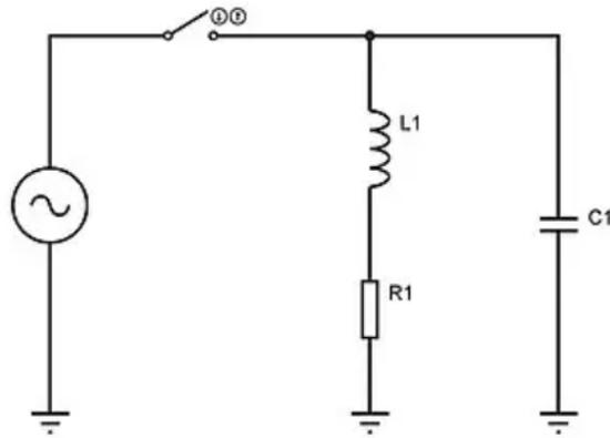
**Figure 7:** power factor correction capacitor with and without inductive load
