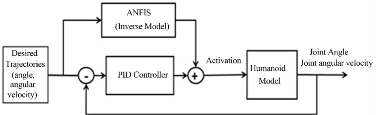
**Figure 5:** A block diagram of ANFIS-PID control system
