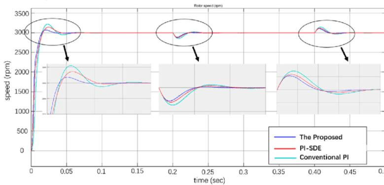
**Figure 6:** Speed reaction curve of BLDC motor of sudden change in load.
