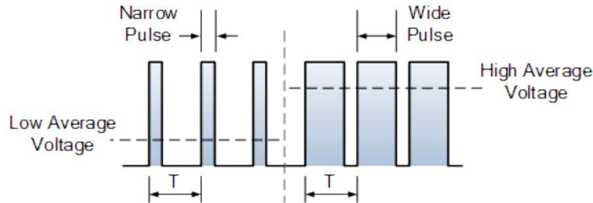
**Figure 4:** Pulse Width Modulated Waveform
